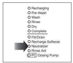
When using the machine for the first time or when the "Add neutralizer" indicator lights, add neutralizer to the storage containers.
